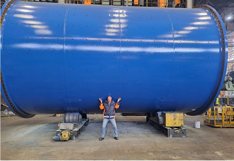
Secondary ball mill - complete
